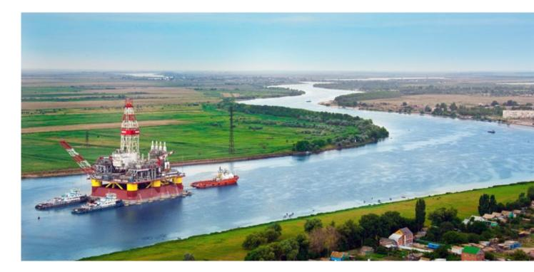
The OTF includes a floater and a single point mooring (SPM). The facility is designed to load 10-12 ths tn deadweight shuttle tankers with crude to ensure the delivery of crude from the Yuriy Korchagin field.
