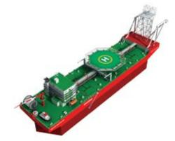
The FSO has double bottom and double sides, habitable deckhouse, machinery space and helipad in the aft of the vessel. She has deadweight of 28,000 tonnes. It measures 132x32 m and with hull-height 15.7 m, and is manned by a crew of 25. The oil is fed to the FSO via the mooring after traveling through a submarine pipeline.
