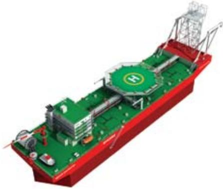
The FSO has double bottom and double sides, habitable deckhouse, machinery space and helipad in the aft of the vessel. She has deadweight of 28,000 tonnes. It measures 132x32 m and with hull-height 15.7 m, and is manned by a crew of 25. The oil is fed to the FSO via the mooring after traveling through a submarine pipeline.
